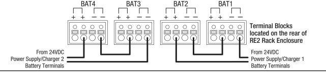
Fig. 1d - Single 24VDC power supply (series parallel connection).
