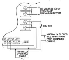
MOM5 module shown with wet and/or dry normally open fire alarm trigger inputs
