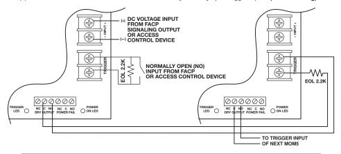
Fig. 4 MOM5 module shown with wet and/or dry normally closed fire alarm trigger inputs
