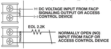
MOM5 module shown with wet and/or dry normally open trigger inputs (Non-Latching):
